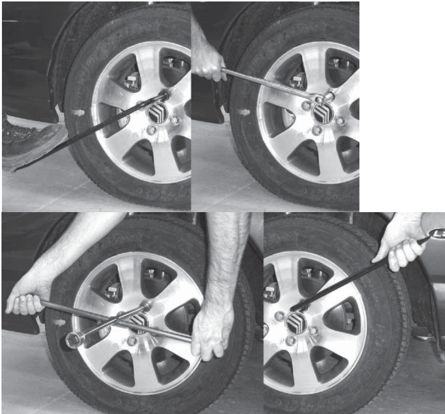
Figure 12-2 Tire changing step 2: Loosen each wheel lug approximately one turn.
