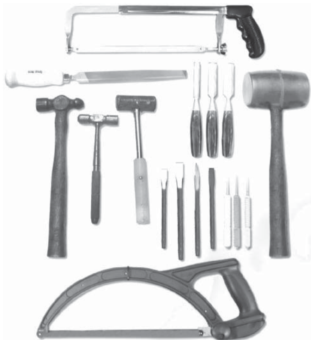
Figure 2-15 Miscellaneous tools that may be needed include a hacksaw, files, punches, chisels, and a ball peen hammer.
