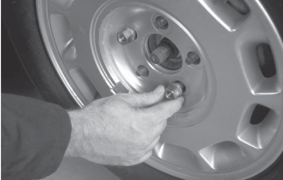
Figure 12-5 Tire changing step 5: Position the spare wheel over the wheel studs. Screw the lugs on by hand and then tighten them with the lug wrench.
