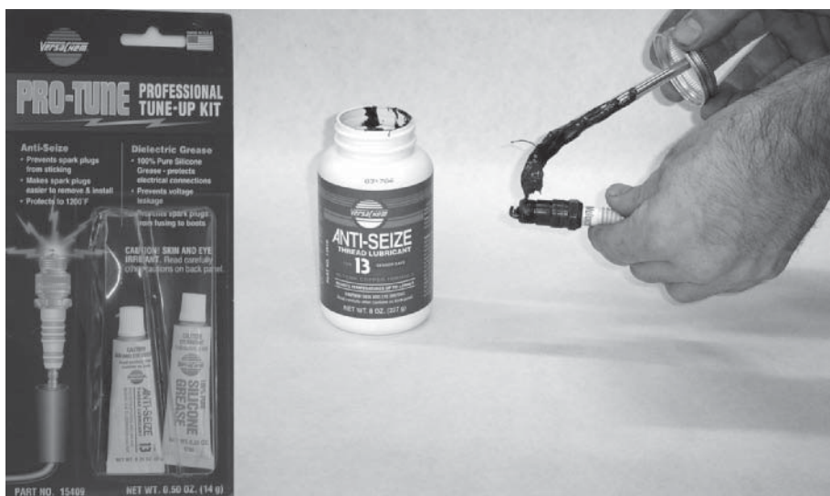
Figure 11-26 A tune-up kit containing silicone grease and anti-seize. Anti-seize is being applied to a spark plug prior to installation.
