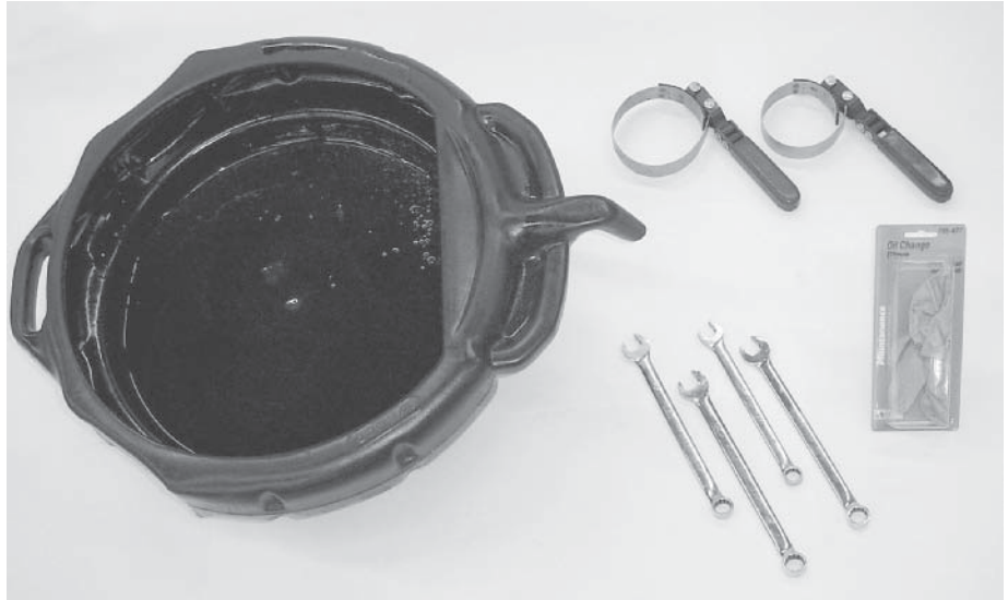
Figure 2–8 Items used for an oil change include a drain pan, oil filter, wrenches, and funnels. Quart containers of oil have a funnel shaped top to aid in pouring.
