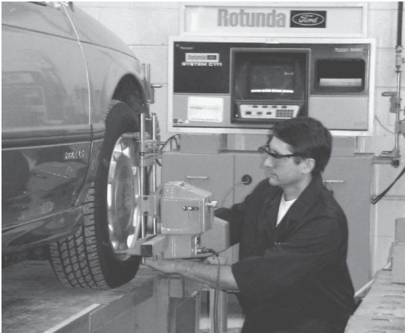
Figure 9-17 An automotive technician performs a wheel alignment using computerized wheel alignment equipment.
