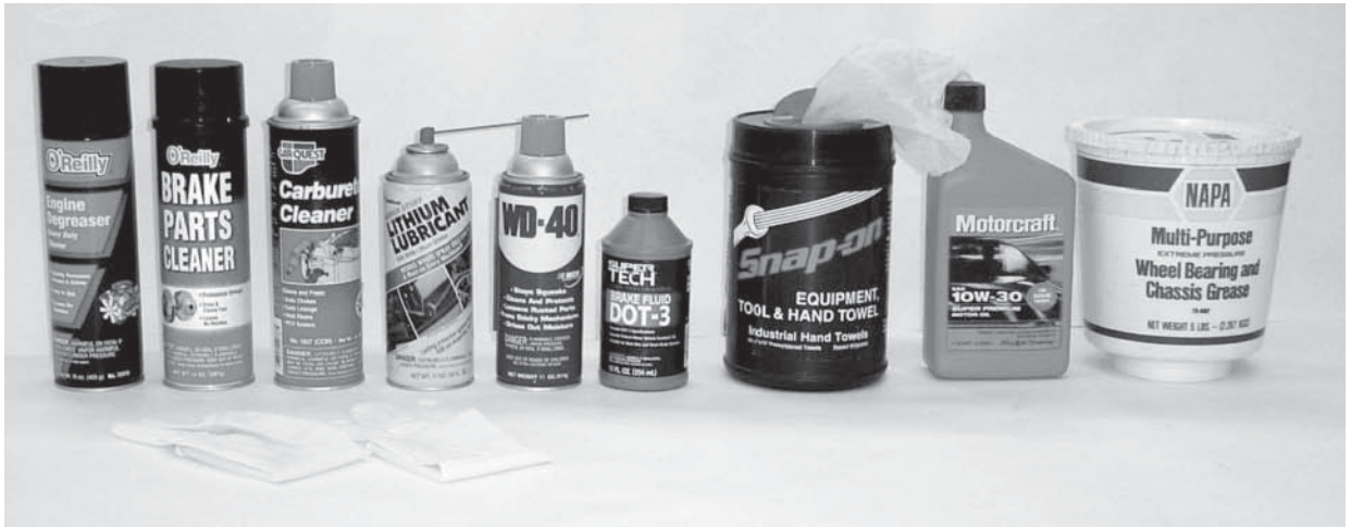
Figure 2-9 A variety of supplies are available for car maintenance, including lubricants, oils, greases, spray cleaners, hand cleaners, hand wipes, latex gloves, and floor dry. These may be purchased at retail parts stores.
