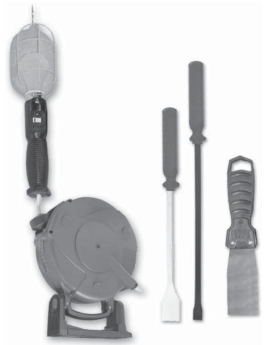
Figure 2-16 Additional shop supplies include a reel-type droplight that can be hung in place while you work on your car. Be sure to use light bulbs designed for this purpose. Other tools include pry bars and gasket scrapers.
