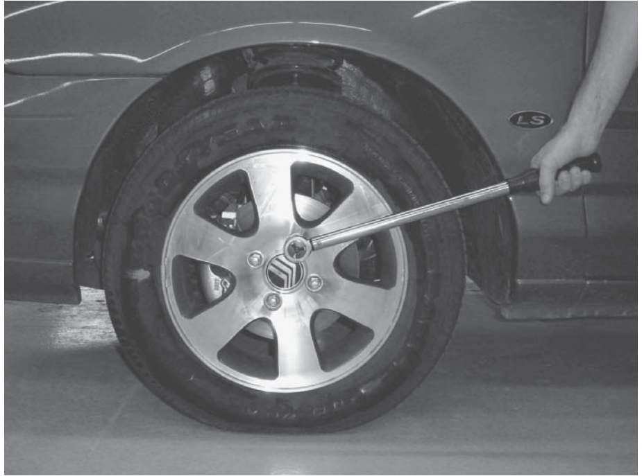
Figure 11-18 Use a click-type torque wrench to tighten wheel lugs precisely.
