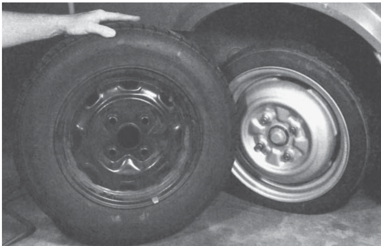
Figure 8-3 Many late-model cars have special, undersized spare tires that are meant for temporary use only.
