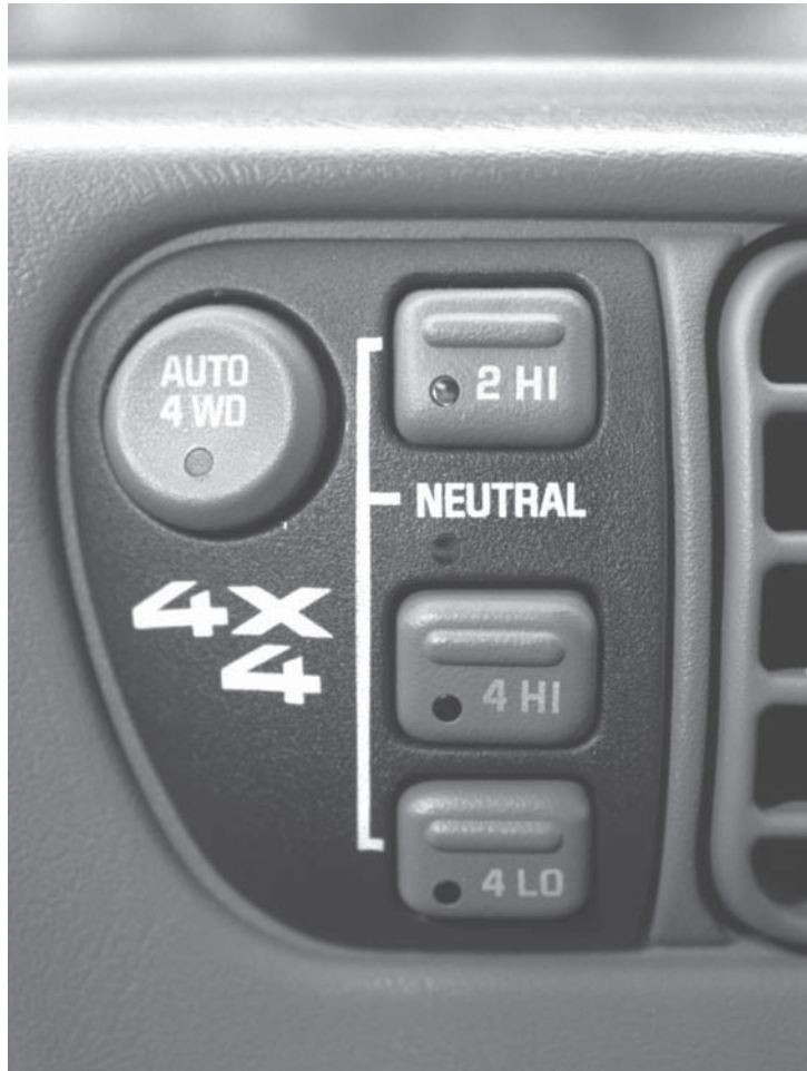
Figure 7-14 Typical controls for controlling a 4WD system on a vehicle.
