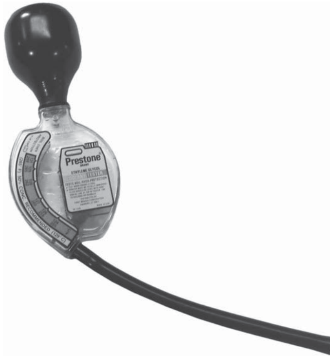
Figure 11-2 A coolant hydrometer can be used to determine the freezing point and relative concentration of the coolant in your car.
