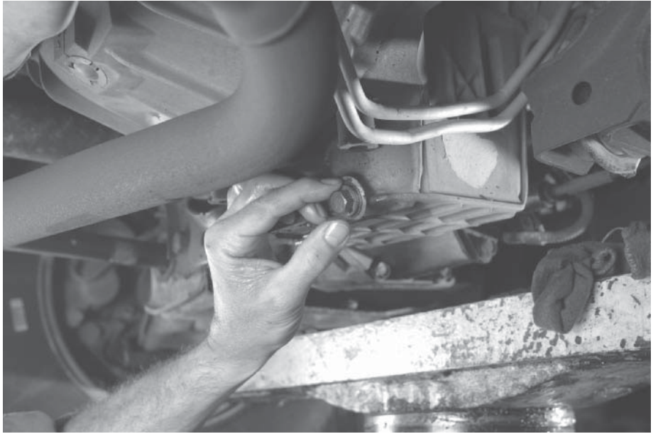
Figure 11-6 Oil change step 3: Clean the drain plug and oil pan, then screw the plug in by hand and tighten it securely.
