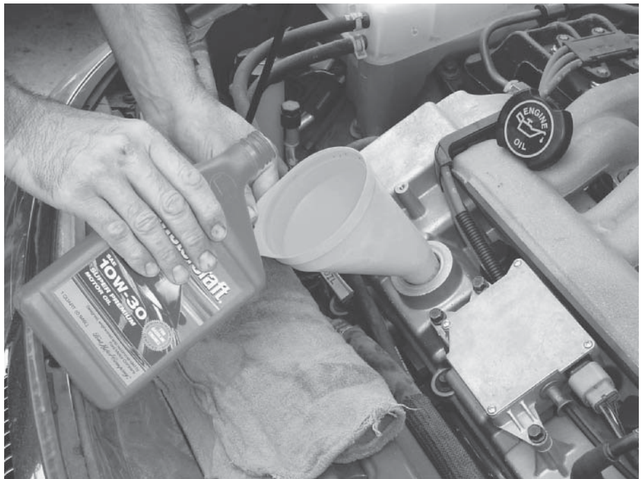
Figure 11-10 Oil change step 7: When the drain plug and filter are tightened securely, add the recommended amount of new oil.
