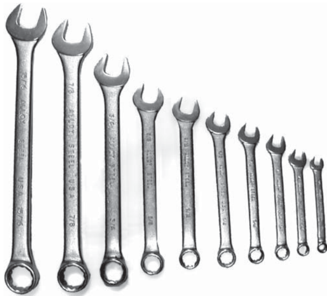
Figure 2-10 Combination wrenches include both an open end and a box end. The wrenches are sized for SAE (Society of American Engineers standard measurements) and for metric sizes. At the top of the photo are examples of box-end wrenches (both ends are box ends) and open-end wrenches (both ends are open ends).
