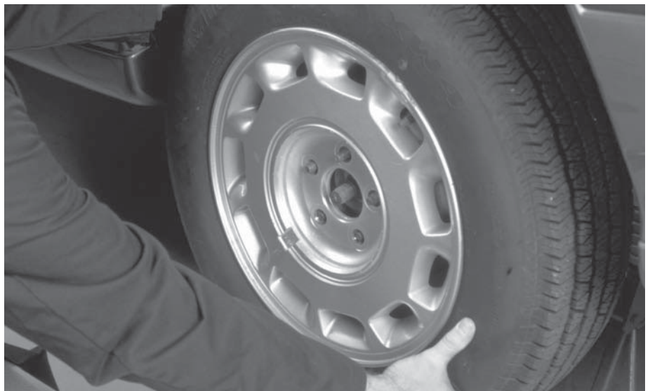
Figure 12-4 Tire changing step 4: Remove the wheel lugs and the tire.
