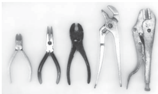
Figure 2-14 Pliers come in a variety of shapes and sizes for a number of different jobs. Shown here, from left, are wire-cutting pliers, long-nose pliers, slip-joint pliers, arc-joint pliers, and locking pliers.
