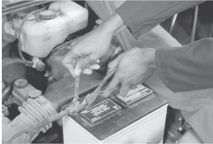
Figure 5-8 Use a backup wrench to hold the battery bolt while loosening the nut on the battery clamp to avoid damaging the battery post.
