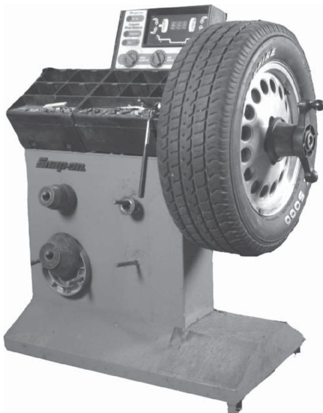
Figure 8-6 A computerized spin balancer called a “dynamic” wheel balancer is used to balance wheels.
