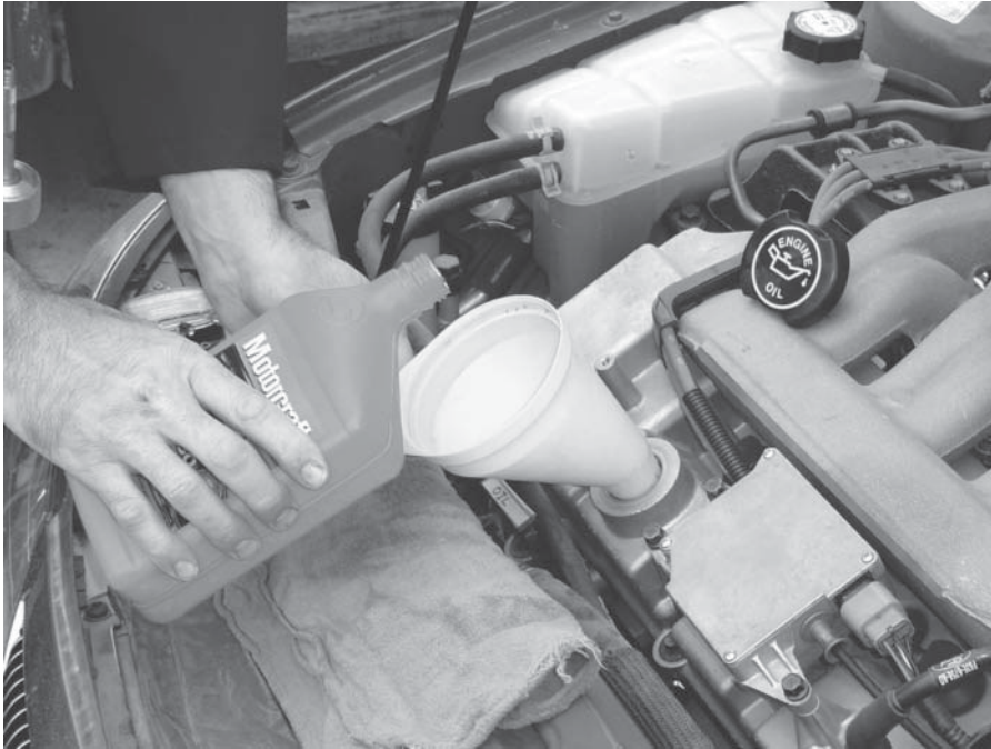
Figure 6-7 You may need a spout or funnel to add oil through the filler hole.
