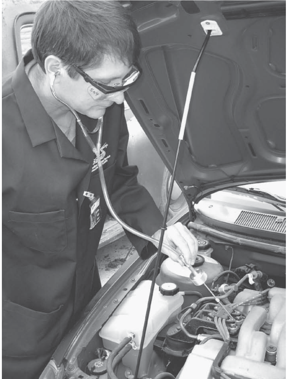
Figure 4-21 A mechanic's stethoscope is used to locate the source of engine and other noises.
