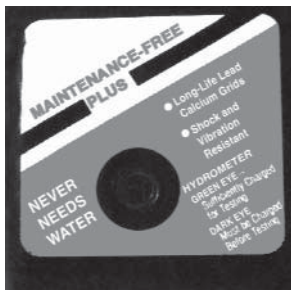
Figure 5-6 A maintenance-free battery is sealed. The condition of the battery is checked by noting the color in the small plastic window.
