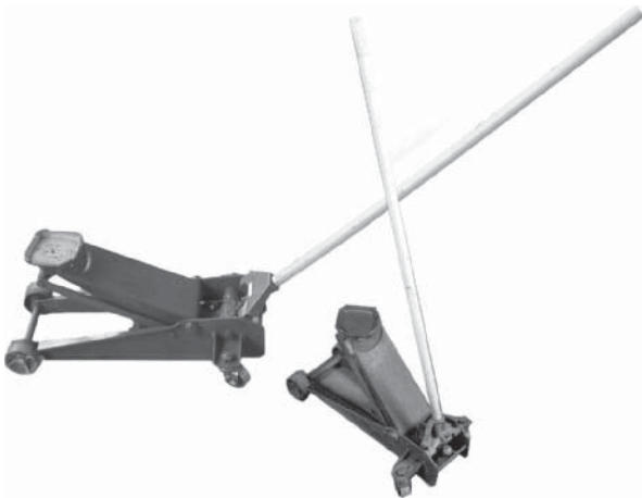
Figure 2-6 A 2¼ ton floor jack may be used to jack up a vehicle. A small portable floor jack may also be used in a garage or carried in the vehicle.
