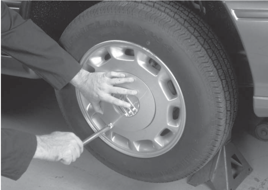
Figure 12-1 Tire changing step 1: Block the diagonally opposite wheel, then remove the wheel cover of the tire to be changed.
