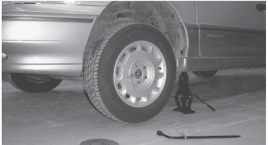
Figure 12-3 Tire changing step 3: Use the jack to raise the tire about an inch off the ground.
