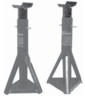
Figure 2-5 For under-the-car work, a set of jack stands should be used to support the car safely. Never place any part of your body under a car supported only by a jack.
