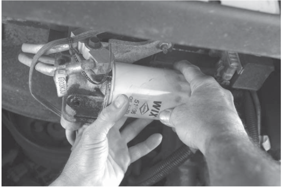
Figure 11-9 Oil change step 6: Screw the new filter on by hand. After the filter contacts the engine, tighten it one-half to three-quarters of a turn more.
