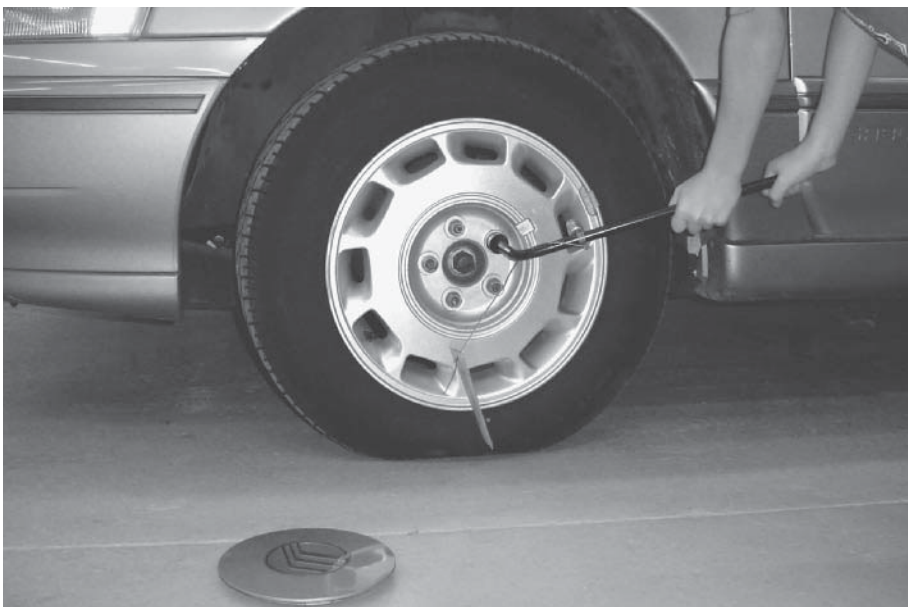
Figure 12-6 Tire changing step 6: Lower the car onto the ground and remove the jack. Then tighten the wheel lugs securely with the wrench.
