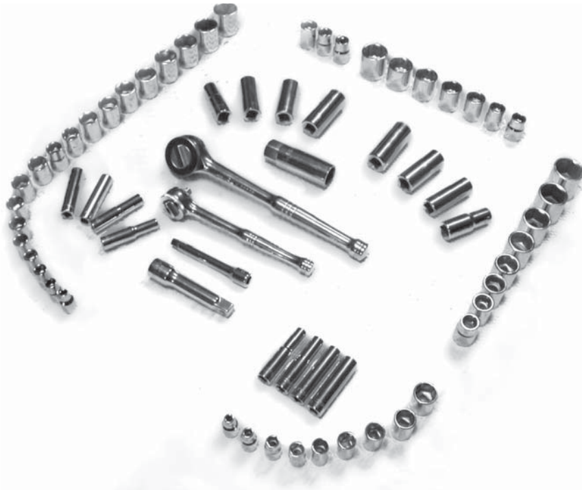
Figure 2-11 A socket set can include extensions, ratchets, and breaker bars (top). These are used to drive, or turn, various types of sockets such as deep well, shallow, and flex sockets.
