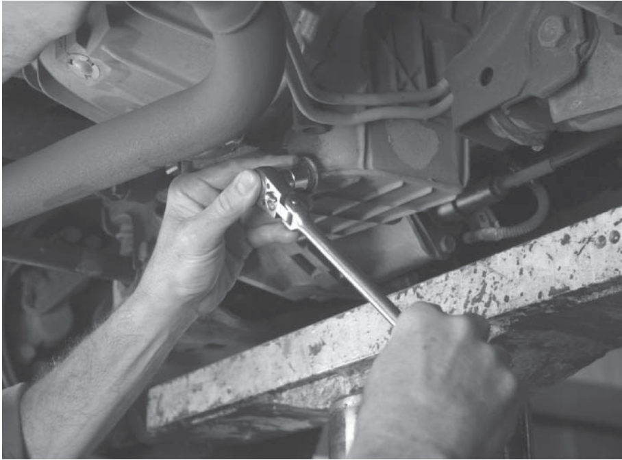
Figure 11-4 Oil change step 1: After raising and supporting the car safely, blocking the wheels, and positioning a drain pan under the car, loosen the drain plug.
