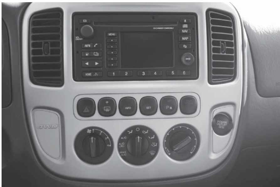
Figure 17-7 This HVAC control knob is color coded to inform the driver which modes are more economical than others.
