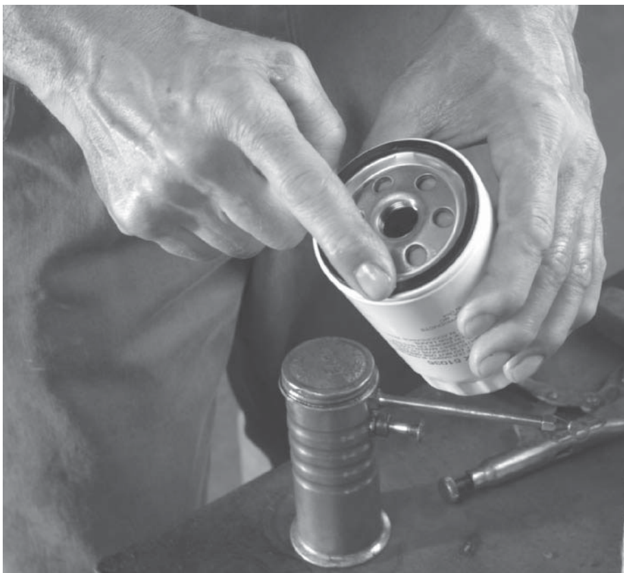
Figure 11-8 Oil change step 5: Rub a few drops of new oil on the new oil filter sealing gasket.
